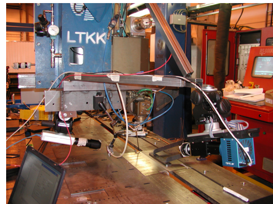
Figure 7. Spectral based monitoring of laser welding.
