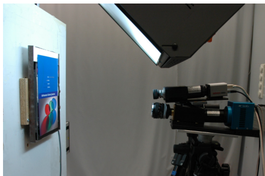
Figure 4. Spectral imaging system from 400nm to 1700nm.
